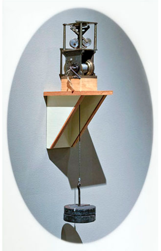
Telescope clock drive with flyball governor, c. 1890
